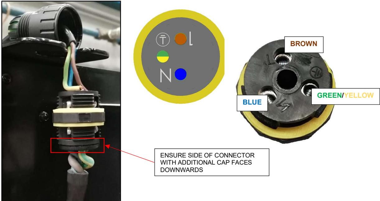
**FIGURE 2, TERMINAL CONNECTIONS**
